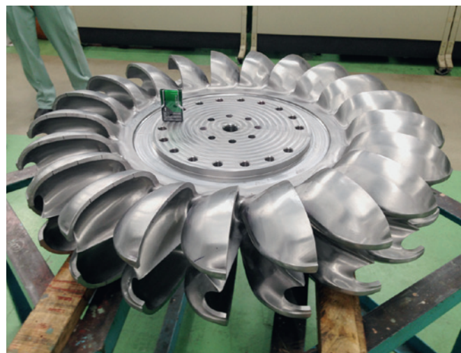
Funama (Japon), la roue monobloc (Q = 586 l/s, Hn = 205 m, Pm = 781 kW)
