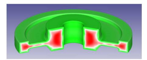
In the disk shown above, the red areas represent tensile residual hoop stress after heat treatment. The green areas are compressive. Stresses in the turbine disk (shown above) were optimized without sacrificing mechanical properties by adjusting the cooling rate during quenching.
