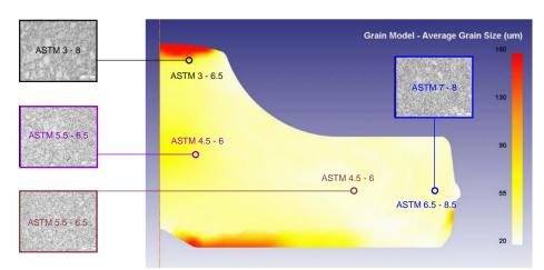
This example, courtesy of Carmel Forge, demonstrates excellent correlation between the model and a production Waspaloy turbine disk forging.
