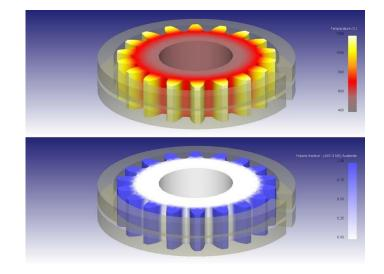
DEFORM also makes it possible to simulate phase transformations in steels. This allows for the prediction of phase, hardness, strength, residual stress and distortion. For example, the spur gear shown above underwent induction heat treatment to yield harder teeth. Induction coils were rotated around the gear to produce uniform heating around the gear circumference. The gear teeth transformed to austenite during heating and subsequently transformed to martensite upon cooling in a quench process.
